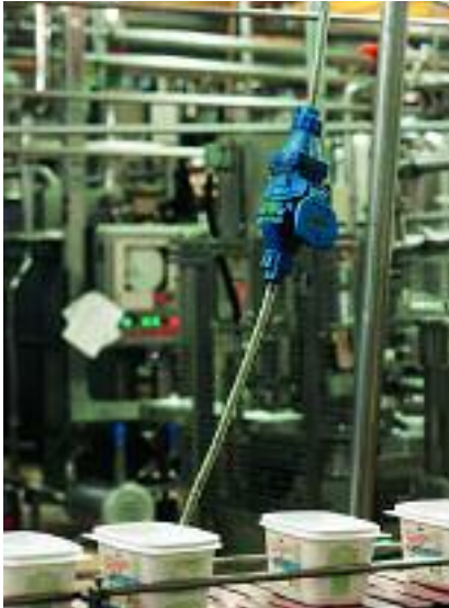
Overhead connections along a production line - dairy industry
